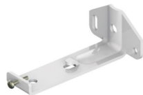
V-014-04E Plated zinc 镀锌 V-014-04F Painted white 烤漆 Wall bracket 89mm Thickness=1.8mm 89蛇形安装架
